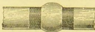
FIG. 35.—Showing the finished wiped joint.
