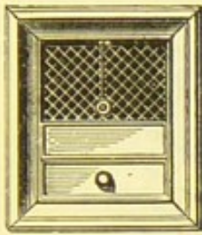
FIG. 76.—Panel air inlet— view from room.
