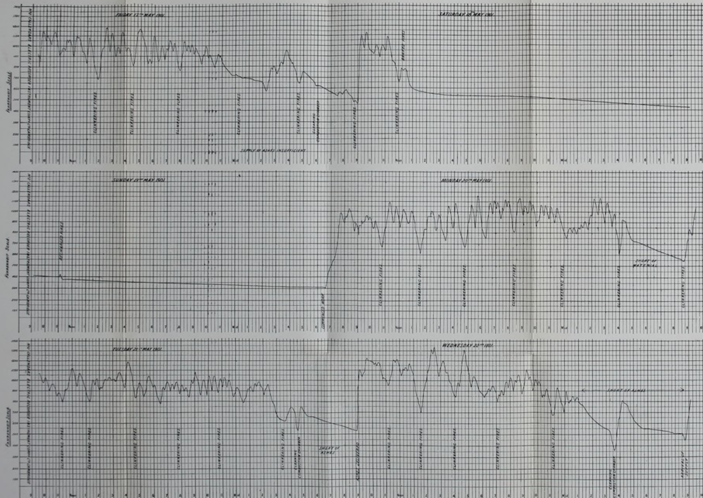
NELSON DESTRUCTOR DIAGRAM OF TEMPERATURE IN DOWNTAKE OF LANCASHIRE BOILER TAKEN WITH A CALLENDAR'S ELECTRICAL RECORDING PYROMETER.
