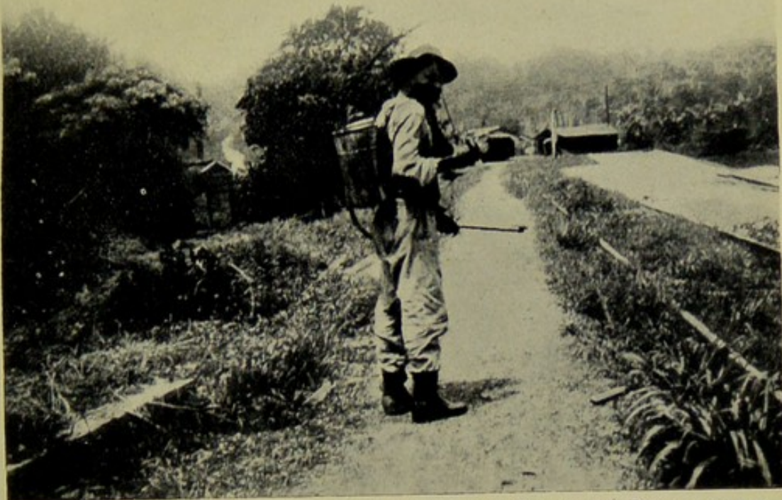
FIG. 23.—ONE OF THE MEN BELONGING TO THE SANITARY DEPARTMENT WITH A KNAPSACK OIL-SPRAYING MACHINE.
