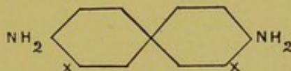
o -dimethyl benzidine (tolidine); o -dimethoxy benzidine (dianisidine); o -dinitro benzidine; o -benzidine disulphonic acid, etc.
