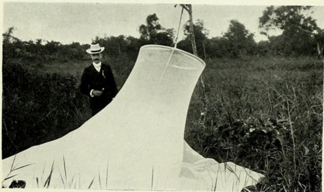
PHOTO. 22.—Net used to estimate number of Anophelines given off by nine square yards of Clairfond Marsh.
