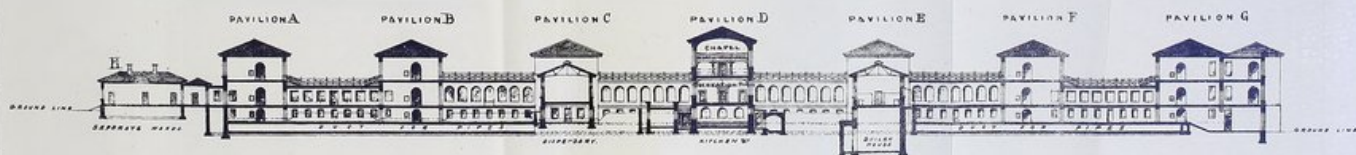
SECTION OF CORRIDOR SHEWING LEVELS OF BOILER-HOUSE, KITCHEN, &c
