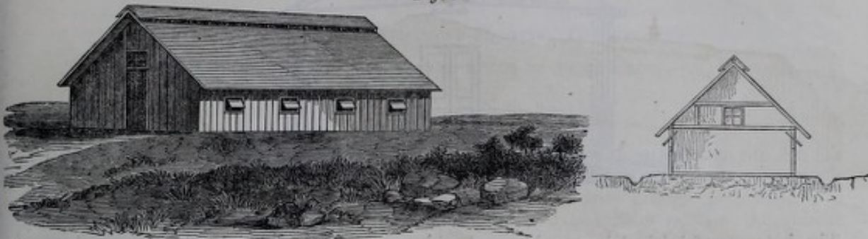
Hut with Site cleared and drained, ridge ventilated, windows, and projecting eaves.
