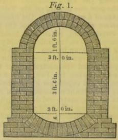
The following figures, 1, 2, are representations of the sewers in the Holborn and Finsbury division of the metropolis, on the same scale as the above. The part in which the joints are marked in the cut is, according to the directions, to be worked in blocks with cement.
