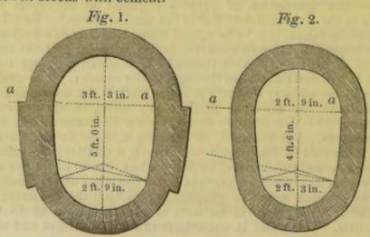
The sides of these sewers form the curves of large radii struck from the centres on the lines aa, the radius for the larger size being about 13 feet,
