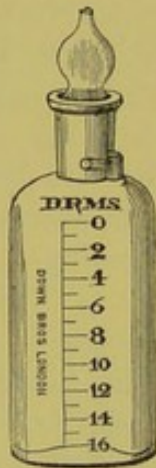
FIG. 25.—GRADUATED DROP-BOTTLE WITH HOLLOW STOPPER.
