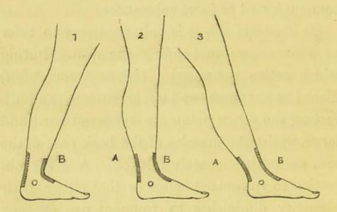
A, represents the back spring, corresponding in form and action to the tendo achillis, or heel tendon; B, the front spring, answering to the peroneii, or those tendons uplifting the front of foot; C. the malleoli, or ankle centre. of a horizontal slip of metal placed in the sole of the foot, and fastened to the leg part by a catgut band, the elastic reaction of which imparts motion to the ankle joint.
