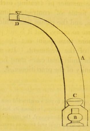
A is the tube, about three feet long, that is commonly used for the hot air bath; a hole is to be cut in its side near the bottom, of sufficient size to admit a copper pot, C, about  $2\frac{1}{2}$  inches deep, and 3 in diameter. This pot is to be supported by wires passing across the tube; it should not touch the sides of the tube, but leave a space of three-fourths of an inch all round; the opening is combined with a certain degree of palsy both of the body and mind. In some in-
