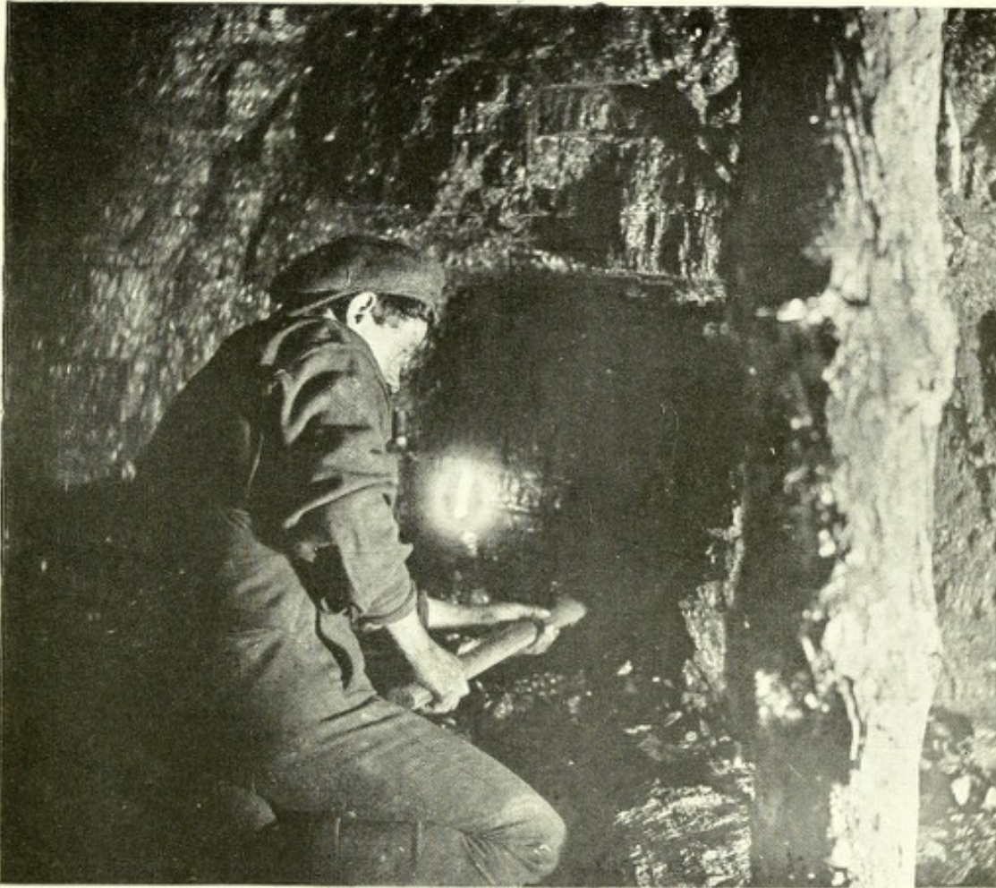
FIG. 18.—BOTTOM HOLING IN A SEAM 4\frac{1}{2} FT. THICK.
