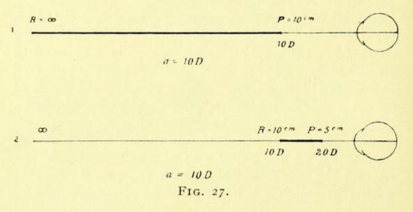
front of the eye, while in Fig. 27 (2), a myopic eye, it is only from 10 cms. (R) to 5 cms. (P) in front of the eye, and yet in each case the same amount of accommodation work is done, which is equal to a lens of 10.
