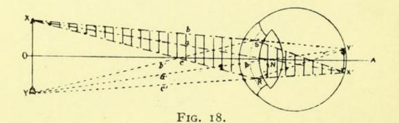
point of this sends out a pencil of divergent rays, and all those which pass into the eye, by the dioptric system, are made to converge into a point on the retina.
