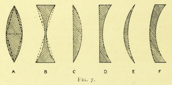
**Lenses.**—If two prisms are placed with their bases in contact, we have roughly a bi-convex lens (Fig. 7, A), and rays of light passing through it are bent towards the base of the prisms—*i.e.*, the centre of the lens; in other words, they converge. If the prisms have their
