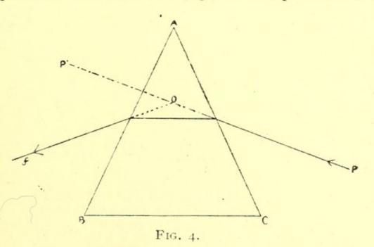
the two plane surfaces. This is called the *refracting* angle, and is written with the sign of a degree after the numeral—thus:  $4^{\circ}$ —which is scratched on the surface of the glass. This is the old, and even up to the present very general, method of numbering prisms.
