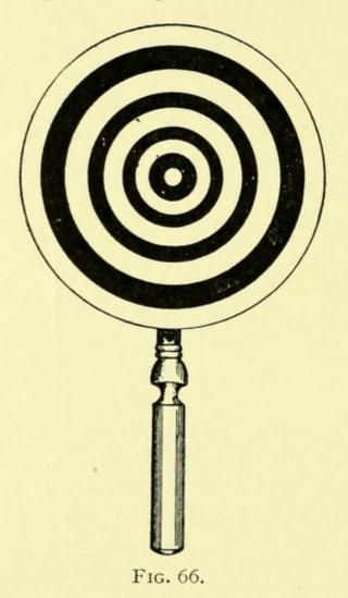
image of the rings is thrown on to the cornea to be examined, the patient being directed to look at the centre. Looking through the central hole, the surgeon sees a diminutive image of the rings on the cornea, and if the latter is normal the rings are round and evenly separated. In regular astigmatism the image appears elliptical, the long axis corresponding with the meridian of least curvature; but when irregular
