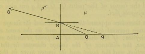
Let QRS be the path of any ray of light, and let RS produced backwards meet the axis in q. Then the angle AQR is equal to the angle of incidence of the ray, and the angle AqR, equal to the angle of refraction. But if  $\mu$ ,  $\mu'$  be the refractive indices of the two media, the law of refraction, expressed in the usual notation, is
