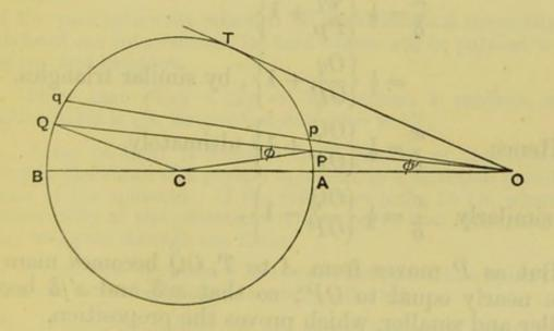
$\sin \phi : \sin \phi' = CO : CP = \mu : 1,$  $\sin \phi = \mu \sin \phi'.$
