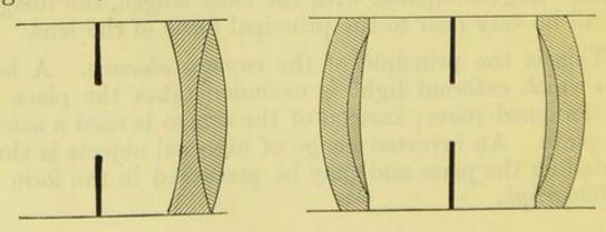
concave lens of flint glass joined to a double convex lens of crown; this combination can be made achromatic and free from spherical aberration near the axis. Such lenses are frequently used now for landscapes and can be made to work up to an aperture f/15 and a field of view of nearly 90°.
