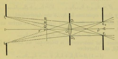
We must now join  $I_1$  to the edges and centre of  $D_1OD_2$  by lines cutting the plane of the object in Q, R and S. Then the plane of the object is divided into rings of different brightness as before. The previous investigation holds, ceteris paribus, and the tangents of the angular fields of view are easily seen to be
