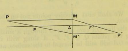
the required point. For one of the rays choose PM, parallel to the axis of the surface, meeting the principal plane at A in M. Then MF' is the corresponding emergent ray. Also, let the ray PF meet the principal plane in M'; this ray will emerge parallel to the axis, so that if we draw M'P' parallel to the axis it will meet MF' in the required point.
