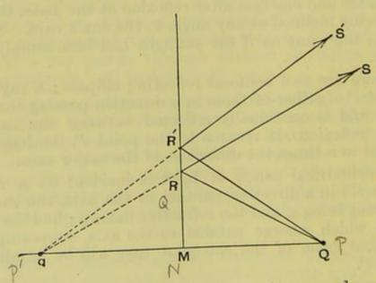
Draw QM perpendicular to the mirror and produce RS backwards to meet it in q; this can always be done, for the lines QM, QR and RS lie in one plane. Then by the law of reflexion it follows that the angle qRM is equal to the angle QRM, and therefore the triangles QRM, qRM are equal in all respects, so that qM = QM.
