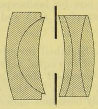
of smaller refractive index than the dispansive lens to which it is cemented, while in the back element the collective lenses are of greater refractive index than the dispansive lens.
