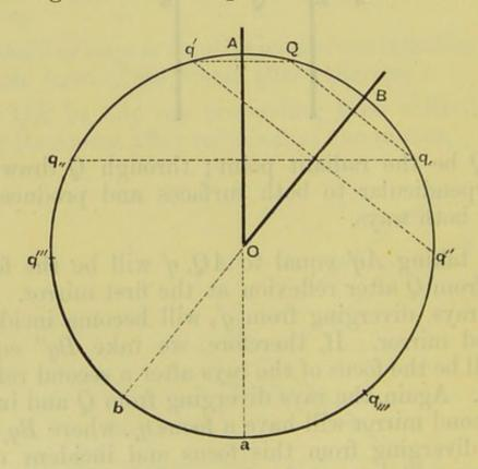
mirrors; and let a perpendicular be drawn from Q to the mirror OA and produced to q', so that Qq' may be bisected by the mirror; then q' will be the focus of the rays after one reflexion at OA. Again, letting fall a perpendicular from q' on OB and producing it to q'', at an equal distance on the other side, q'' will be the focus of the rays after a second reflexion, and so on. In like manner we find
