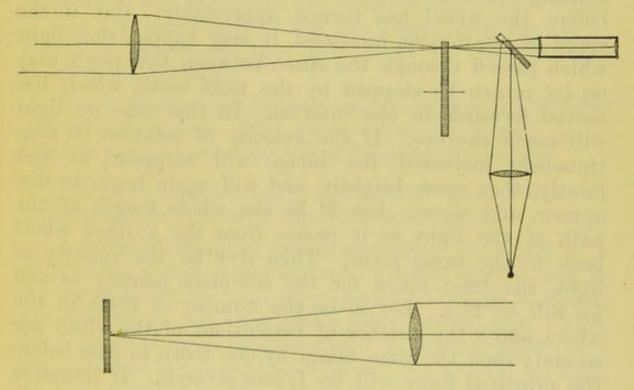
the other telescope; in this instrument a plate of glass, inclined at an angle of 45° to the axis of the telescope, is placed between the eye-piece and the principal focus of the object-glass. Light is admitted through the side of the instrument and reflected down the tube by the
