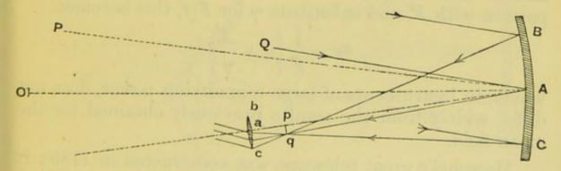
The arrangement of the mirror and eye-lens is shown in the figure. BAC is the large spherical reflector, AO being its axis, and O its centre; AP is the axis of the tube and Aa the axis of the eye-lens, and these two lines are equally inclined to AO, the axis of the mirror. Bq, Aq, Cq, are three rays which are brought to a focus at q by
