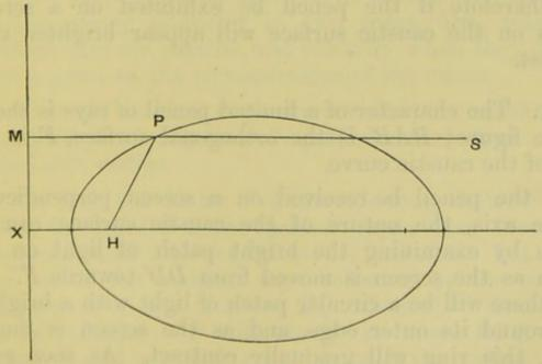
But  $\mu SP + \mu PM$  is also constant. Choose the plane MX so that this constant quantity may be equal to c; then  $\mu'HP = \mu PM$ , and therefore the surface is formed by the revolution of a conic whose focus is H and directrix MX, about its major axis.
