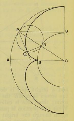
cide with B. Now as Q begins to move, the point of contact R is for an instant fixed, so that the motion of Q is perpendicular to QR; and therefore the reflected ray PQ touches the curve described by Q. This is true whatever the position of the point P. The locus of Q is an epicycloid, and this is the caustic curve required.
