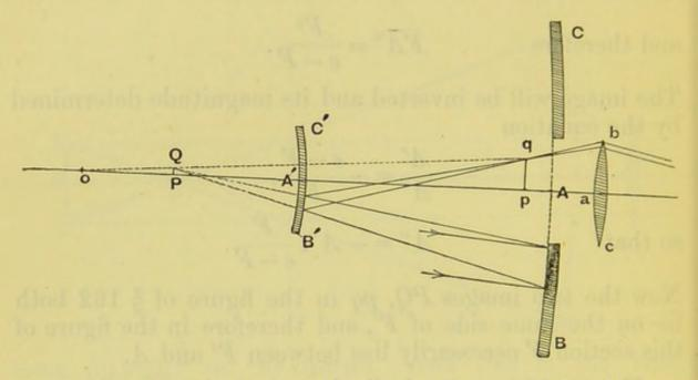
of what had been done in England. Cassegrain's telescope only differs from Gregory's in having its small mirror convex instead of concave, and placed between the large mirror and its principal focus. The arrangement of the mirrors and images is shown in the figure.
