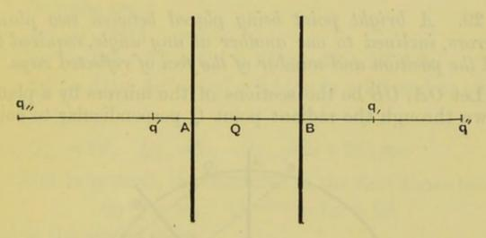
Let Q be the radiant point; through Q draw a line AQB perpendicular to both surfaces and produce it indefinitely both ways.
