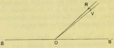
transmit red rays copiously to the eye, and similarly for the other colours. Thus to the eye there will appear a series of coloured arches with the violet rays innermost The effect of the rays which strike the eye with greater deviation, will be to light up the cloud within the bow with faint light, while no light will reach the eye from drops lying outside the bow.
