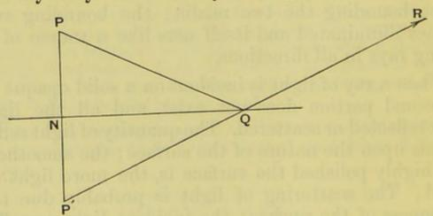
struction. If P be any point on the incident ray PQ, and if from P a perpendicular PN be drawn to the reflecting plane and be produced to P' so that P'N is equal to PN, then in the triangles PNQ, P'NQ, the two sides PN, NQ are equal to the two sides P'N, NQ, each to each, and the
