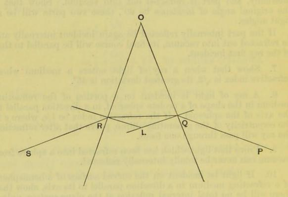
In the first case the rays PQ and RS lie on the sides of the normals away from the vertex, and therefore the deviations both at ingress and egress will be away from the edge of the prism.
