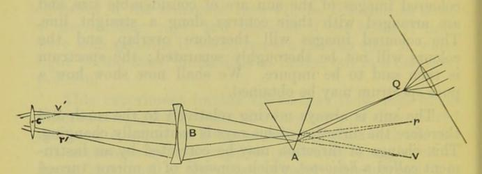
v', where rBr', vBv' are straight lines. The colours are now perfectly separated, but the spectrum v'r' is very small, so that it needs to be magnified before it can be accurately measured. The spectrum is therefore viewed through another lens or eye-piece (also corrected for chromatic dispersion). The two lenses constitute an ordinary astronomical telescope. If therefore the rays from the prism be received on a telescope, by focusing the telescope we shall be able to see a pure spectrum.
