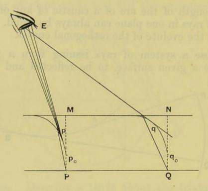
this caustic which will meet the eye, and then these lines will bound the part of the pencil which traverses the air; if we join the points where these tangents meet the surface to P, the joining lines will bound the pencil as it passes through the water. The two tangents to the caustic meet at the point of contact of either of them, very nearly. Thus to an eye outside the point P appears to be at p.
