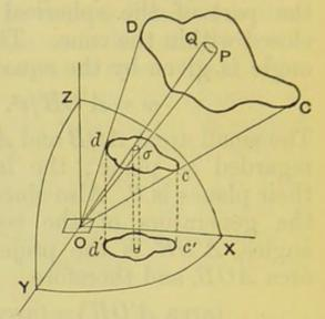
By addition we arrive at the following method of determining the illumination of a small area at O due to any finite bright surface.
