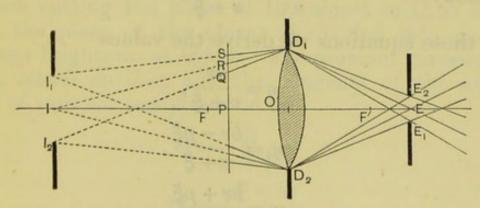
$I_1II_2$  is the incidence pupil, and the field of view is limited by the lens-aperture. Join  $D_1$  to the centre and edges of the incidence-pupil, cutting the plane of the object in Q,
