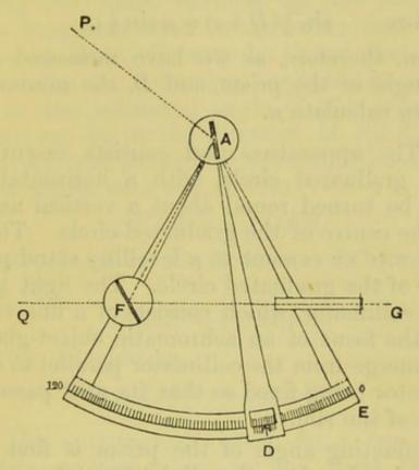
The inclination of the mirrors may be read off the graduated scale. If the arc be graduated so that every half-degree may be read as a degree, the reading will give the angular distance between the two points without any further calculation.
