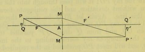
Referring back to the geometrical construction (§ 47) for finding the point P' conjugate to a given point P, it follows from the similar triangles PQF, M'AF that
