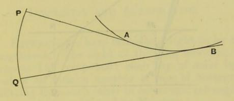
any number of times. For each ray, form the function  $\Sigma\mu\rho$ , and let  $V=\Sigma\mu\rho$ . Let the final medium be of refractive index  $\mu$ , and let  $V=V_0$  be the value of the reduced path for an orthogonal curve in this medium, say the curve PQ. Let AB be any arc of the caustic, and let PA, QB be the rays touching at A, B. Then the arc AB = QB - PA, by the properties of evolutes.
