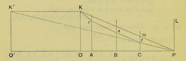
122. When an object PL is seen through any number of lenses, the breadth of the principal pencil where it falls on the eye at O, is to its breadth at the object-glass (that is, the lens nearest to the object) as the apparent distance of the object to its real distance from the object-glass.
