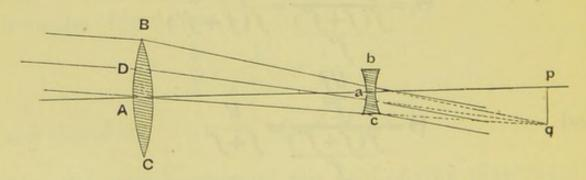
144. This telescope, called after its inventor, Galileo, was the first whose construction was explained on theoretical principles. It differs from the astronomical telescope chiefly in the form of its eye-glass, which is a double concave lens, and is placed between the object-glass and its principal focus. A pencil of light diverging from the
