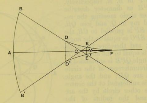
and a bright spot is developed in the centre. When the screen is at EE' the circle of light reaches its minimum; this circle is called the *least circle of aberration*. When this position is passed, the outer boundary expands again though the bright ring still contracts. Beyond F, no part of the screen is specially illuminated.
