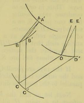
therefore the same as along ABCDE. Take away the common parts; then if  $\mu$ ,  $\mu'$  belong to the initial and final media, there remains the equation,  $\mu A'B + \mu'DE' = \mu AB + \mu'DE$ . But, since AB is normal to the surface AA', A'B = AB ultimately, and therefore, DE' = DE; that is, EE' is perpendicular to DE. The same may be proved for every point E' near E, and thus the surface EE' near E is perpendicular to the ray DE, and by similar reasoning to every other ray of the system.
