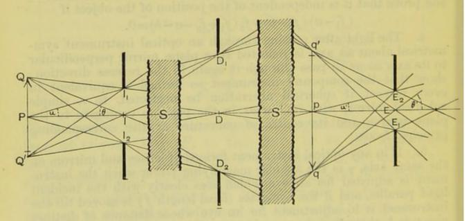
Suppose that  $D_1DD_2$  represents a diaphragm placed anywhere in an optical instrument, and denote the systems of lenses which lie in front of the diaphragm (that is on the side nearest the object) by S, and that which lies behind it by S'. Let the image of the diaphragm formed by the lens-system S be  $I_1II_2$ , and that formed by the system S',  $E_1EE_2$ . Then every ray which in the instrument
