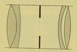
It consists of a cemented achromatic pair as the first element, with a back pair, separated by a small interval. The back pair may be moved nearer or further away from the front pair by a rack and screw-head. It is clear that for portrait lenses rapidity is a great advantage. At the same time very accurate definition is not necessary except in the centre of the picture; it is regarded as an advantage that there should be considerable diffusion or softness in the details of the background.
