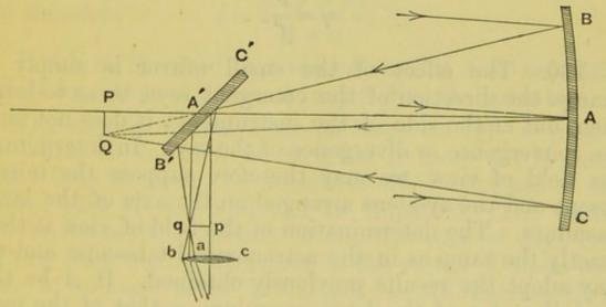
The arrangement of the mirrors and the eye-lens is shown in the figure. BAC is the object-mirror, B'A'C' the plane mirror, and bac the eye-lens. Rays BQ, AQ, CQ are reflected by the large mirror to a focus Q, where PQ is the
