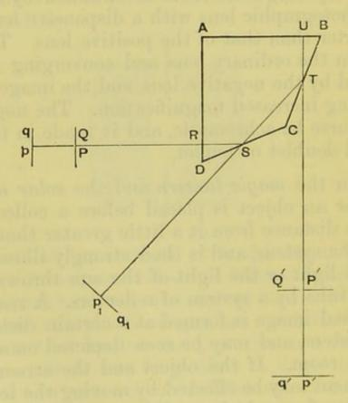
$q_1p_1$  will be again reflected at the surface CB and another image q'p' will be formed. Finally when the rays proceeding from q'p' are refracted again into the air, they
