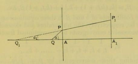
In the figure, suppose that  $QAA_1$  represents the axis of the system, QP the incident ray,  $Q_1PP_1$  the course of the ray after one refraction, produced backwards to meet the axis in  $Q_1$ . Then  $AQ = b \cot \alpha = b\mu/\beta$ . This relation may be expressed in the form  $\mu/AQ = \beta/b$ . In exactly the same manner it may be shown that  $\mu_1/AQ_1 = \beta_1/b$ .
