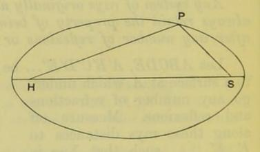
of a single reflexion at a curved surface, we choose our surface such that SP + PH may be the same for all paths, and therefore the surface must be an ellipsoid of revolution whose foci are S and H.
