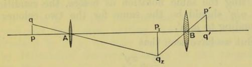
For let x, x' be the distances of the object and its first image in front of, and behind, the first lens, y', y the distances of the first and final image in front of, and behind, the second lens, respectively, and let  $\eta$ ,  $\eta_1$ ,  $\eta'$  be the linear magnitudes of the object and its images. Then the following ratios must hold:
