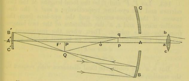
smaller mirror, and ab the eye-glass. Rays proceeding from a point of the object are reflected at the large mirror and are brought to a focus in Q, where PQ is in the principal focal plane; also Q and the corresponding point of the object lie on the same line through the centre of the large mirror. After passing Q, the rays diverge and are
