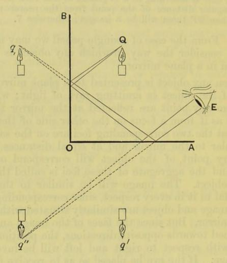
the two mirrors, and the rest dotted. Finally, we draw the pencil from Q to the points of the section of the last pencil made by the mirror OB. Rays issuing from Q are reflected first at the mirror OB, then again at the mirror OA, and finally enter the eye in the same direction as if they proceed from an object situated at q''.
