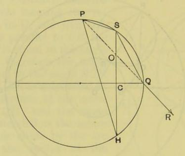
fracted ray. Describe a circle about the triangle SHQ, and let QR be produced backwards to cut the circle in P; then PQ bisects the angle SPH. Let  $\phi$  be the angle of incidence and  $\phi'$  the angle of refraction at Q; then the angle  $POS = \phi'$ , and  $\phi = \angle HSQ = \angle HPQ = \angle SPO$ .
