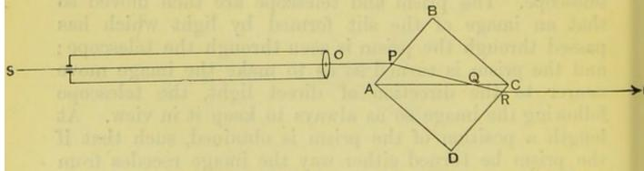
an illuminated slit, admitting light. The rays, incident on the prism, pass through it and emerge in a direction parallel to that of incidence, so long as the angle of incidence on the fluid layer is less than the critical angle. The compound prism is turned about so as to increase the angle of incidence on the fluid; as soon as the critical angle is reached, the light is totally reflected
