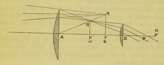
Let A, B be the centres of the lenses, AF the focal length of the lens A; then since AF = 3f', AB = 2f', the point F is also the principal focus of the lens B. Since q'p' is in the focal plane of the lens B,  $Bp' = \frac{1}{2}AB$ . Also, since p, p' are conjugate foci with respect to the lens A,
