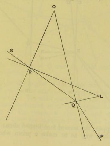
other angle, OQR, being acute. Then the ray SR lies on the side of the normal towards the vertex, so that the corresponding deviation is towards the vertex, while at Q the deviation is away from the vertex. But the angle of refraction at Q is greater than that at R, the former being the exterior angle of the triangle QRL and the latter an interior angle. Hence the deviation at Q is greater than that at R, so that on the whole the deviation is away from the vertex.
