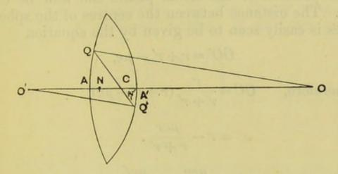
There exist two points on the axis of the lens, which are most useful in the determination of the positions of conjugate foci, and corresponding incident and emergent rays. They are a pair of conjugate foci, such that any incident ray passing through one of them, will emerge in a parallel direction through the other. These points are called the *nodal* points, and also from another property which will be pointed out later, the *principal* points of the lens.
