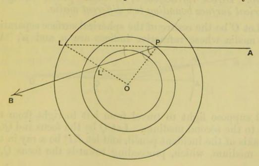
Let the original medium in which the ray moves have a refractive index  $\mu$ , and the sphere an index  $\mu'$ . With centre O describe two other spherical surfaces whose radii are respectively  $r\mu'/\mu$  and  $r\mu/\mu'$ . Produce the incident ray to meet the first sphere in L; join OL cutting the second sphere in L', then PL' is the refracted ray.
