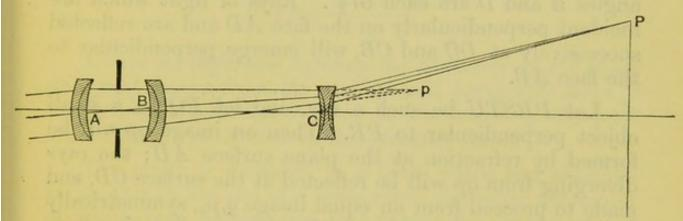
The necessary length of focus is obtained by uniting an ordinary photographic lens with a dispansive lens of focal length shorter than that of the positive lens. The pencils issuing from the ordinary lens and converging to a focus are received by the negative lens, and the image is thrown back, causing increased magnification. The negative lens must of course be achromatic, and is made in the form of a cemented doublet or triplet.
