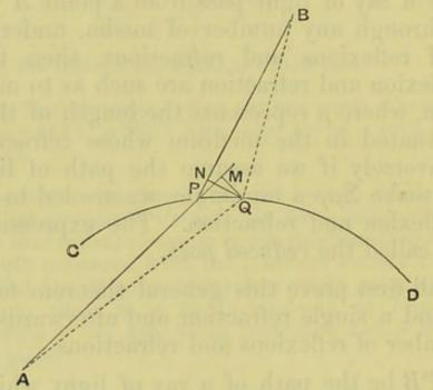
Let the angles of incidence and refraction at P be  $\phi$ ,  $\phi'$ ; then  $\mu \sin \phi = \mu' \sin \phi'$ . Let AQB be a consecutive path; it will be sufficient to take the case when Q is in the plane APB.
