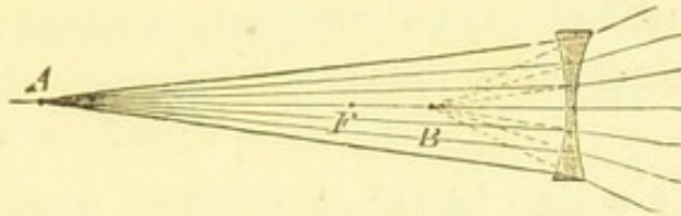
Action of a concave lens on convergent and divergent rays.
