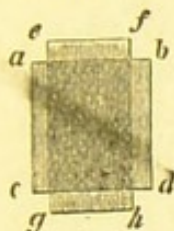
Tourmaline plates placed parallel to each other.
