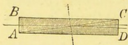
Double prism of Quartz.
