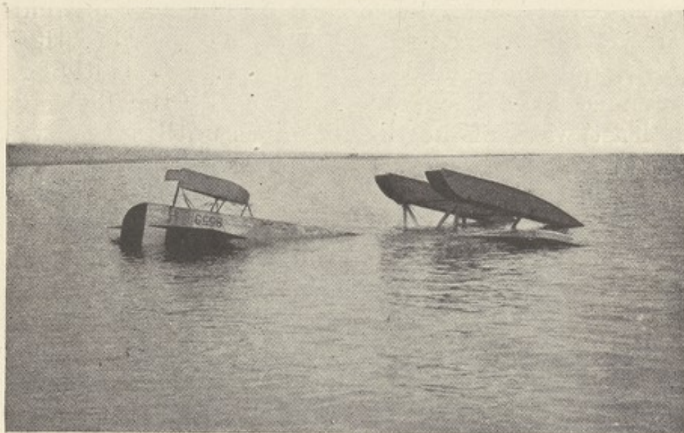
FIG. 16.—Showing a sinking seaplane with under surface of main floats now uppermost.
