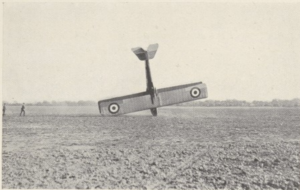
PLATE 12A.—Showing result of flattening out too late. Aeroplane photographed in the act of overturning—occupants uninjured.
