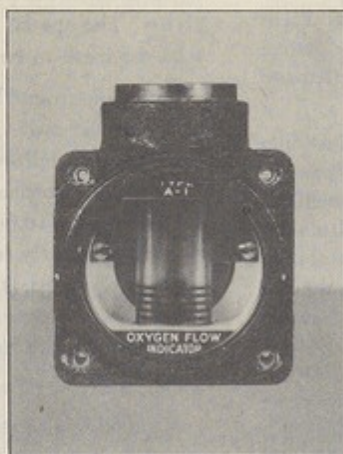
Figure 53—Two views of the type A-1 flow indicator (ball in glass tube).
