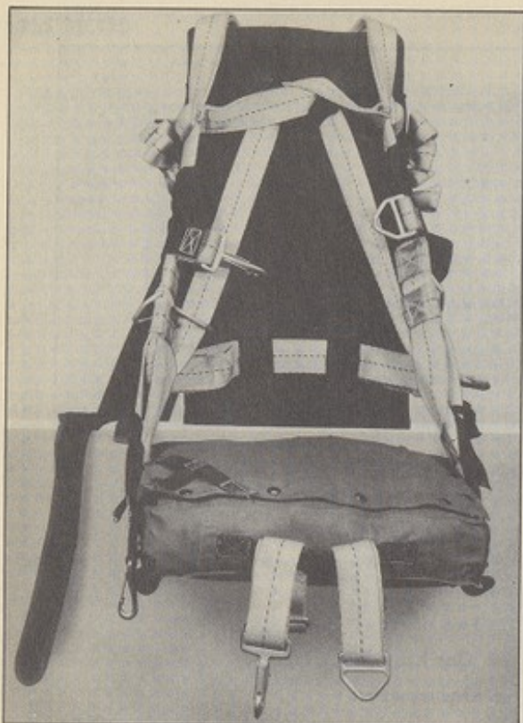
Figure 68—The one-man pneumatic life raft pack as fitted to a back type of parachute. It is attached outside the harness.
