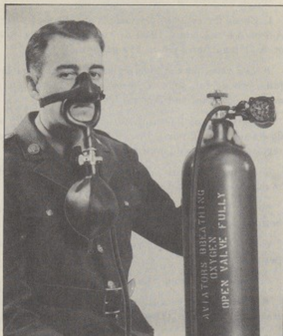
Figure 36—Subject wearing a type A-7 oxygen mask, connected to cylinder of oxygen.
