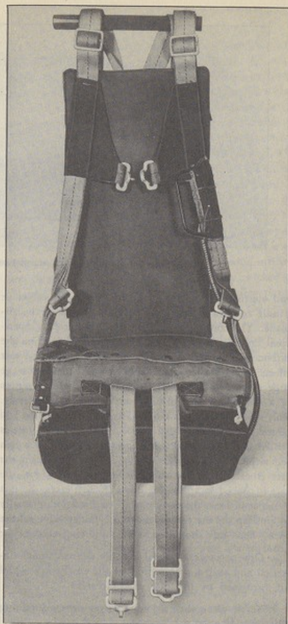
Figure 69—The one-man pneumatic life raft pack as fitted to a seat-type parachute, front view.
