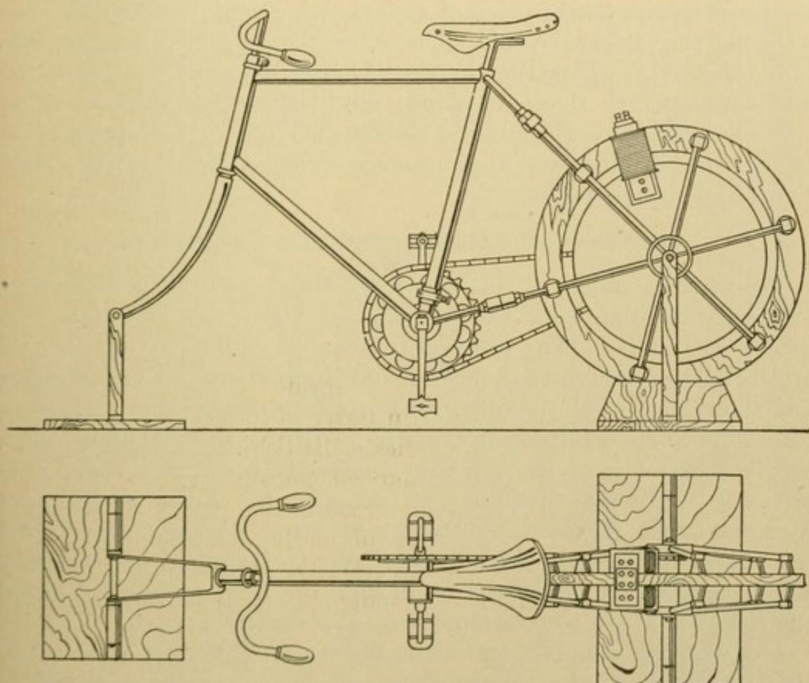
FIG. 1.—The bicycle ergometer.
