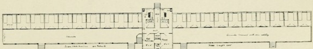
No. 84.—Iowa State Sanatorium, Oakdale, Ia. H. F. LIEBBE, ARCHITECT. LEAN-TO, 240 FEET LONG. VIEW OF FRONT AND SIDE ELEVATION AND FLOOR PLAN. CAPACITY, 40 PATIENTS. ESTIMATED COST, $8,000. (See illustrations 24, 29 and 103 for further description of this institution.)
