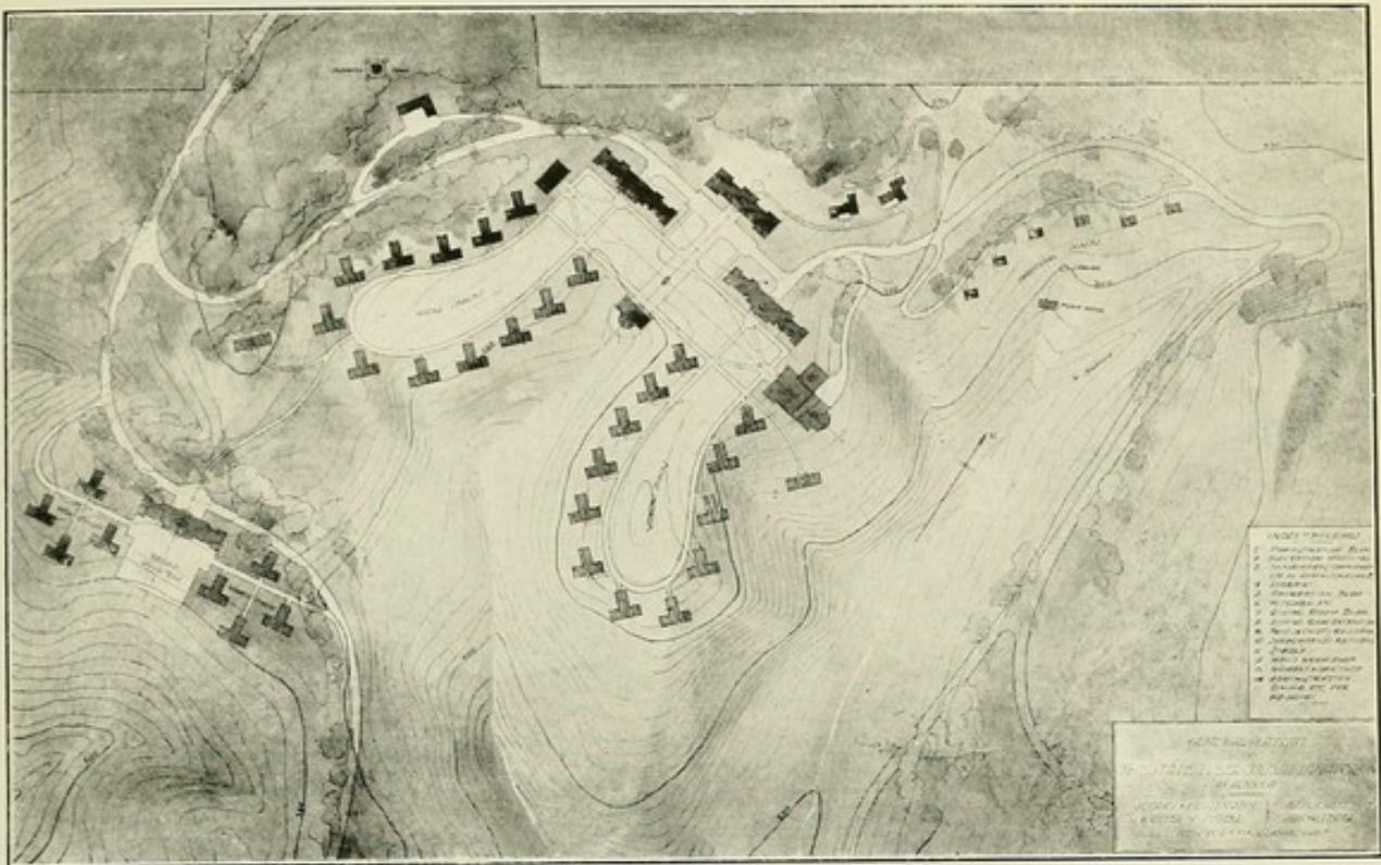
No. 4.—Georgia State Sanatorium, Alto, Ga. SCOPES & FEUSTMANN, AND WALTER W. JUDELL, ASSOCIATED ARCHITECTS. BLOCK PLAN SHOWING THE CONTOUR LINES AND THE METHOD OF GROUPING THE LEAN-TOS ON TWO PROMONTORIES IN FRONT OF THE ADMINISTRATION BUILDING. NOTE THE NEGRO QUARTERS ON THE LEFT OF THE ILLUSTRATION IN THE FOREGROUND. CAPACITY TO BE 400 PATIENTS. ESTIMATED COST, $175,000. (See illustrations 65 and 78 for further description of this institution.)
