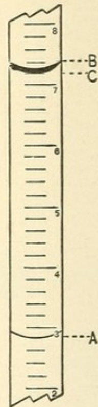
FIG. 40. — Fat in Neck of Test Bottle. Reading should be made between A and B not between A and C. (Wing.)
