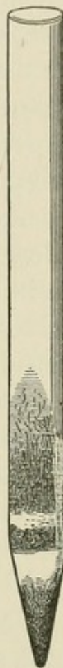
Ordinary reduction-tube, with two sublimes; the upper, brownish-black; the lower, the pure metal in an annular deposit.
