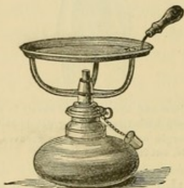
Spirit-lamp and tray for heating (annealing) gold foil.
