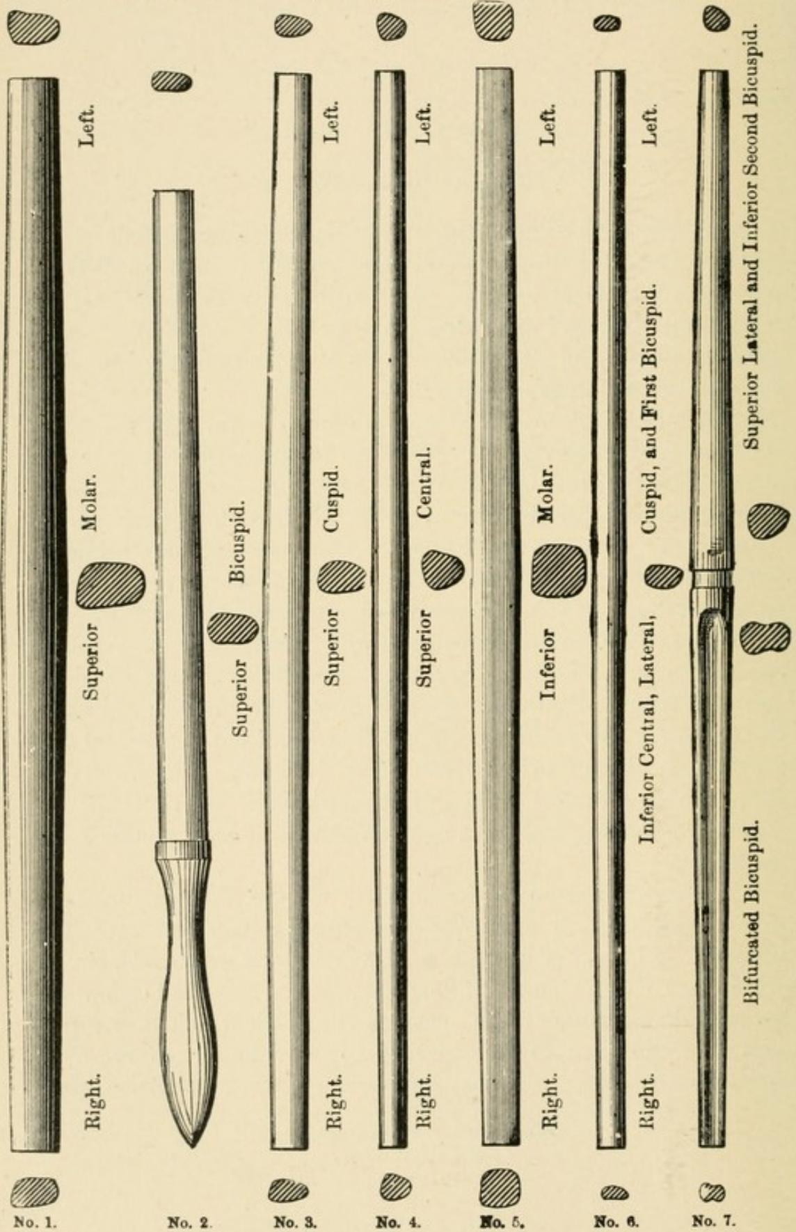
size, the longest instruments being nine inches in length. The cross-sections show the shapes and proportionate sizes at the greatest and least diameters. The long taper permits the most minutely accurate adjustment of the collars.
