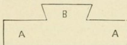
crown, the ends being placed at the side opposite to that where the collar will be joined to the bridge if the space permits. The collar is then removed and the ends soldered together (Fig. 434). The collar is readjusted on the crown, and the part at B, Figs. 434 and 436, bent down over the occluding surface, so that it nearly meets the collar section A. On the outside of the collar a slightly narrower strip of gold clasp plate, No. 30 (Fig. 435),
