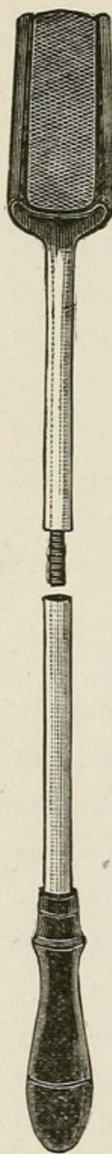
FIG. 42. HOUSE'S REVERSI- BLE RASP, JOINTED.
