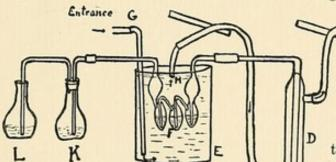
and D is a condenser kept at a temperature of from  $40^{\circ}$  to  $50^{\circ}$  C. E is a beaker into which the water enters at G, is heated to a temperature of from  $40^{\circ}$  to  $50^{\circ}$  C. by a Bunsen burner, **C** and is drawn off by means of a siphon
