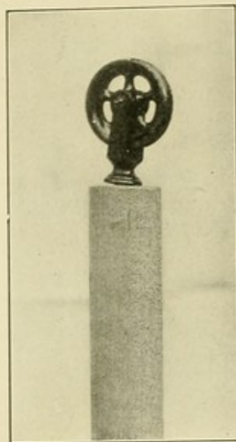
Fig. 401.—Pulley arranged on broom-handle to be fastened at foot of bed for carrying extension cord.
