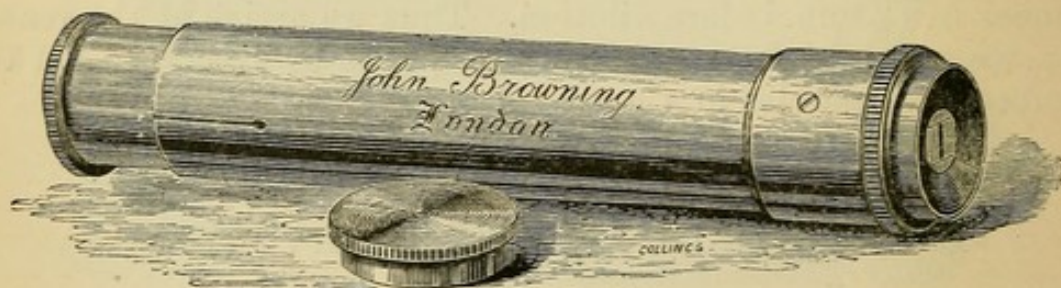
FIG. 18.—Browning's Straight-Vision Spectroscope.
