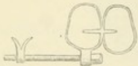
Figure 49.—Showing the form of band and screw used in moving the bicuspid. The nut was fixed in the vulcanite plate.
