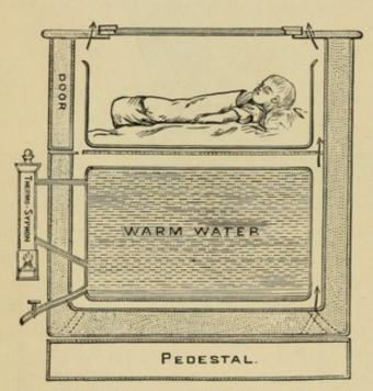
Fig. 143.—Section of hospital incubator. (Tarnier.)
