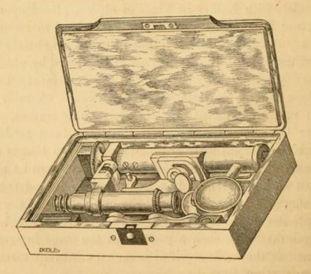
Fig. 4.—Gruby's compound pocket microscope, exactly one-half the real size.
