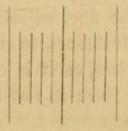
Five ruled spaces in an eye-micrometer, corresponding to one of those above, and each consequently equal to the 1-5000th of an inch.
