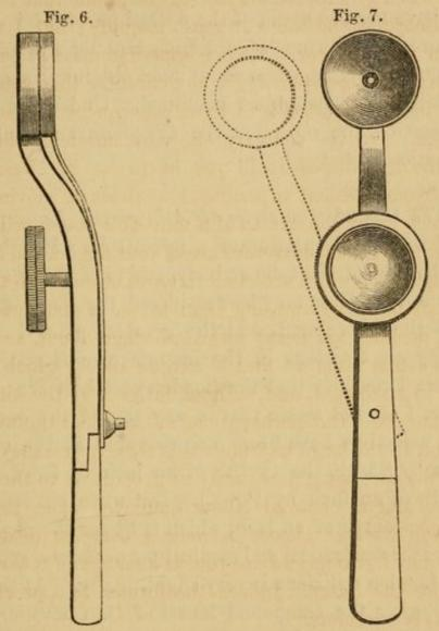
GAIRDNER'S SIMPLE CLINICAL MICROSCOPE.—Fig. 6, a lateral view of the instrument. Fig. 7, a front view, showing in outline the posterior glass separated and turned aside.
