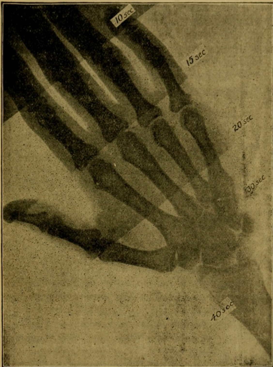
SUCCESSIVE TRIAL EXPOSURES from 10 to 40 seconds, 9" spark coil. Cossor's Bianodal Tube warmed down to 3\frac{1}{2} " alternative spark. Edwards' Kathodal Plate (whole-plate size). Distance between tube and plate 12". Metol Quinol Developer applied for 20 minutes as described in text.
