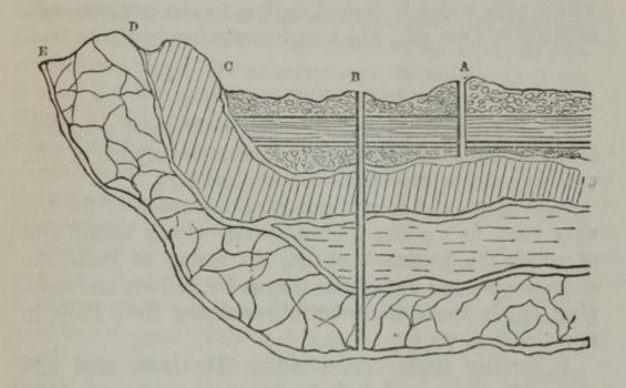
This illustration represents a vertical section of the earth, at a given locality, exhibiting the geological formation of the region, and the subterraneous sheets of water.
