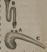
four times its bulk of water. Immediately the mixture begins to boil or effervesce with violence, and air-bubbles rush abundantly from the beak of the retort. Allow them to escape for a little, till you suppose that the common air which previously filled the retort has been displaced by the newly generated air. Then place an in-
