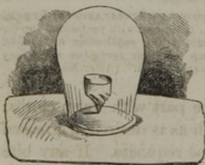
A view of the Cup when exhausted by the combustion of Alcohol applied in it by means of the paper cone, showing the position of the latter. The upper end is the part which burns, after being moistened in the alcohol. (After Nature.)
