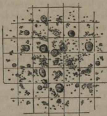
Microscopic Appearance of Heavy Carbonate of Magnesia.
