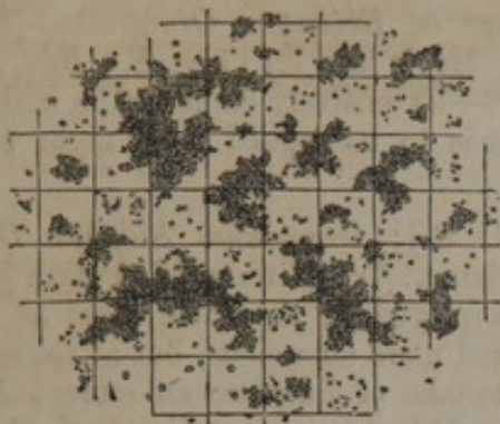
Microscopic appearance of pure precipitated sulphur. (The micrometer squares are equal to those seen in Figs. 58 and 60.)
