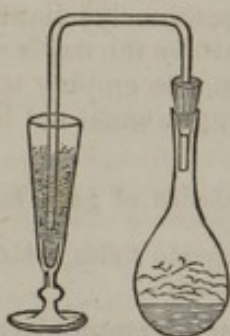
Mode of passing Hydrosulphuric acid through an arsenical solution.
