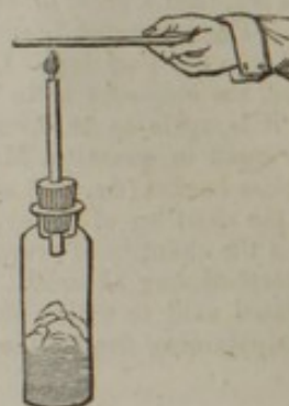
Simple mode of applying Marsh's Test.
