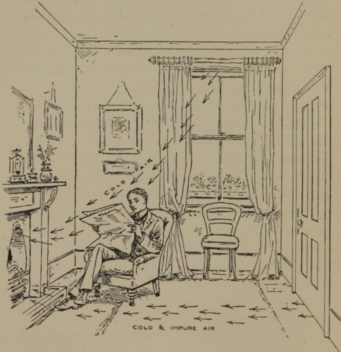
BADLY VENTILATED ROOM
