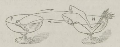
No. 2. Both legs were now placed in one glass, and the portion of the spine attached by the nerves in the other glass, and connection made with the poles of the battery. The direct current was allowed to traverse the nerves for thirty minutes, when the muscles ceased to contract, whether the circuit was made or broken. Upon reversing the poles, the inverse current now flowing upon the nerves, the muscles again contracted, showing conclusively that the diminished excitability
