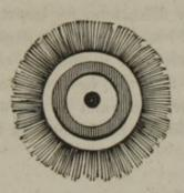
Common sand, ground pumice stone, emery, the debris of a grindstone, or crocus, may be used on the brush with water, and the final polish may be given with a similar circular brush and dry whiting.
