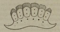
44. When the plaster has been thoroughly dried, which may be done in an oven, provided the operator be in haste, or over a fire in a ladle, provided the degree of heat used be not sufficient to recalcine the plaster, the piece is ready to be soldered.
