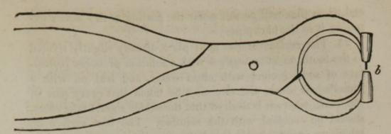
The shears (a) must be strong; and the plate-punch (b) of sufficient material to sustain the force required to perforate the
