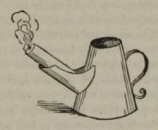
The orifice of the spout into which the wick is inserted, should be at least three-fourths of an inch in diameter, and the vessel capable of containing a quart or more of oil.
