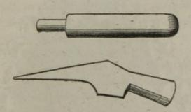
The sharp and broad edge of the hammer must be applied with repeated strokes and a skilful hand to the lingual side of the inner edge of the plate until it shall effect the object to the extent desired. There is but one method of avoiding the necessity of this operation, which is to pare away the plaster cast upon which the metal casts are to be made, along the inner edge of the plate, so that the plate in being struck between the me-
