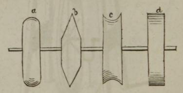
Although these edges, corners, planes and curves remain long with little apparent change, which is by no means true of any other wheels used for the purpose excepting copper ones; yet it must be evident that constant use will more or less change those original forms, unless the mode of grinding upon them shall be calculated to preserve the primitive shapes; a point to which ordinary ingenuity will direct the attention of the artist.
