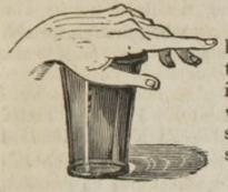
IF, as represented in this figure, the air be exhausted from a vessel, covered by the hand, its removal will be found almost impracticable: for, supposing the opening, which the hand closes, to be equal to five square inches, the pressure on it will be seventy-five pounds.
