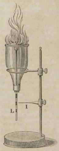
THE inflammation of ether, upon the surface of water, as represented in the following figure, does not cause any movement in the liquid included in the bore of the thermometer at L, although the bulb is within a quarter of an inch of the flame. Yet the thermometer may be so sensitive, that touching the bulb, while under water with the fingers, may cause a very perceptible indication of increased temperature.
