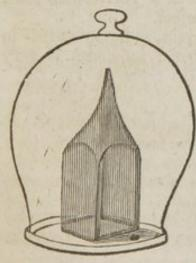
If a thin square bottle, so sealed, that, while unbroken, the contained air cannot escape, be placed within the receiver of an air pump, the exhaustion, of the receiver, will cause the fracture of the bottle.
