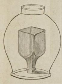
THE mouth of a square bottle, being placed over the hole in an air pump plate, so as to be sufficiently tight for exhaustion, a few strokes of the pump, by withdrawing the air from the interior, causes the bottle to be crushed with violence.
