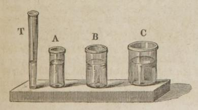
LET the vessels A B & C be supplied with water through the tube T. The water will rise to the same level in all. Of course the resistance made by the water in each vessel to the entrance of more of
