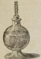
ABOUT the wick of a spirit lamp, a fine wire of platina is coiled, so as to leave a spiral interstice between the spiral formed by the wire; a few turns of which should rise above the wick.
