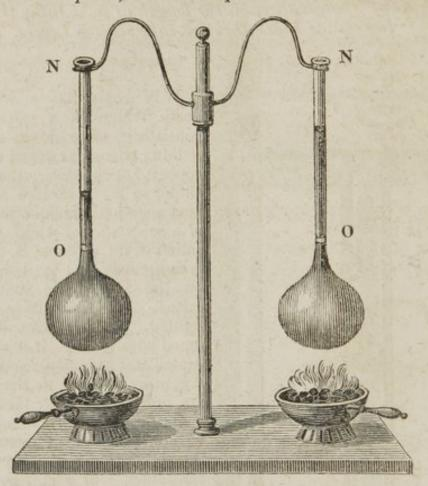
Let two globular glass vessels, as above represented, with long narrow necks, as nearly as possible of the same size and shape, be supplied severally, with water and alcohol, excepting the necks from NN to OO. Under each vessel, place equal quantities of charcoal, burning with a similar degree of intensity. The liquids in both vessels will be expanded, so as to rise into the necks; but the alcohol will rise more than the water.
