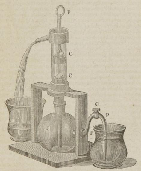
A little suction pump is constructed, with a chamber, CC, of glass, which permits the action of its piston, P, and valves to be seen. Below the pump is a hollow glass globe filled with water. This globe communicates with the pump, by a tube visibly descending from the lower part of the pump, through an aperture in
