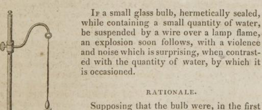
Supposing that the bulb were, in the first instance, merely filled with steam, without any water in the liquid form, the explanation of this phenomenon would be comprised in the theory of expansion given page 2. In that case, the effort of the steam to enlarge
