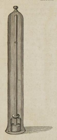
It has been shown, that in a tube void of air, a mercurial column may be supported nearly at the height of thirty inches; and this has been alleged to result from the pressure of the atmosphere on the surface of the mercury without the tube.
