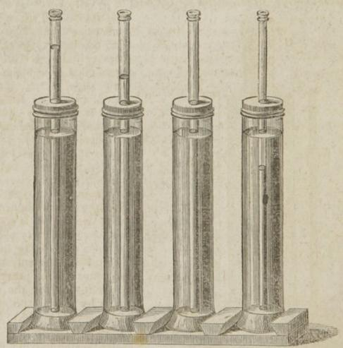
LET there be four jars, each about four inches in diameter, and more than thirty inches in height—severally occupied by mercury to the depth of about two inches. In the axis of each jar, let a
