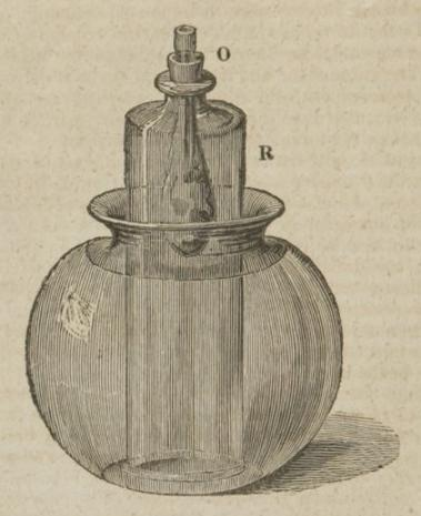
A TALL receiver, R, with an orifice, O, like a bottle, is placed in a globe of water, so that about two-thirds of the receiver is occupied by this liquid, the remainder with air—whilst a bladder is
