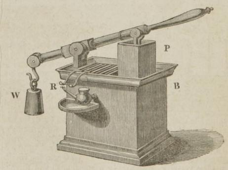
THE preceding figure represents an instrument for igniting a lamp, by means of a galvanic discharge, from a calorimetor; for an
