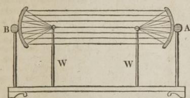
THE object of the model represented A by this diagram, is to explain the mode in which two mirrors operate, in collecting the rays of heat in one focus, and in concentrating them in another.
