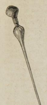
By means of a bag of caoutchouc, fastened upon the neck of a glass bulb, with a long tapering perforated stem, as in the annexed figure, an instrument may be constructed, of great use in a
