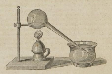
A MATRASS, situated as in the above figure, and containing a small quantity of water, being subjected to the flame of a lamp, the water will soon, by boiling, fill the matrass with steam. When this is accomplished, bubbles of air will cease to escape from the neck of the matrass, through the water in the vase.
