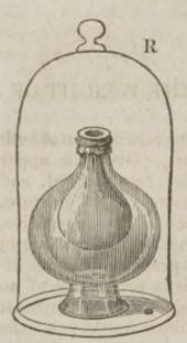
The mode, in which the air occupying but a small part of a vessel may be rarefied, so as to occupy the whole cavity, is shown by the experiment represented in the annexed engraving. A bladder is so suspended within a vessel included in a receiver, R, that the cavity of the bladder, communicates, through its own neck and that of the vessel, with the cavity of the receiver; while no such communication exists between the receiver, and the space between the bladder and the inside of the vessel.
