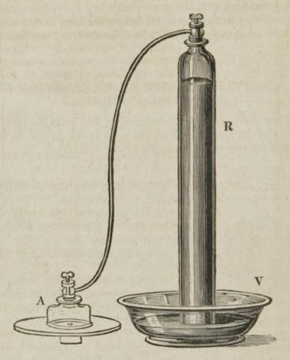
Rs a glass receiver about 33 inches in height, with a perforated neck, into which a brass gallows screw is cemented; so that by means of the flexible pipe communicating with the air pump plate A, he receiver may be exhausted. The mouth of the receiver being immersed in mercury, in the vase, V; as the exhaustion proceeds, the metal rises in the receiver, until it reaches more or less nearly to the height, at which it stands in a Torricellian tube, accordingly as the pump is more or less perfect.
