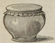
LET there be a glass vessel, open at both ends, as in this figure. Over the upper opening, let a bladder be stretched, and tied, so as to produce an air tight juncture. For every square inch of its superficies, the bladder, thus covering the opening in the vessel, sustains a pressure of about fifteen pounds: yet this is productive of no
