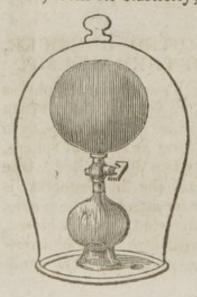
This power, of any portion of included air to extend itself, in consequence of removal of pressure, is illustrated in another way, by subjecting to a highly rarefied medium a gum elastic bag, its orifice being previously closed, so as to be air-tight. The bag will swell up in a most striking manner, in proportion to the diminution of power in the air without the bag, to counteract the reaction of the air within it.
