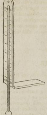
THE thermometers used in laboratories, are usually constructed so as to have a portion of the wood, or metal, which defends them from injury, and receives the graduation, to move upon a hinge, as in the accompanying figure.
