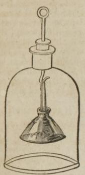
Let a portion of water, just adequate to cover the bottom, be introduced into the vessel, represented, in the subjoined drawing, as hanging within a receiver. Over the water, let a stratum of ether be poured, from an eighth to a quarter of an inch in depth. If, under these circumstances, the receiver be placed on the air pump plate, and sufficiently exhausted, the water freezes.
