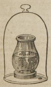
WATER heated to ebullition in a glass vessel, having ceased to boil in consequence of its removal from the fire, is made to boil again in an exhausted receiver.
