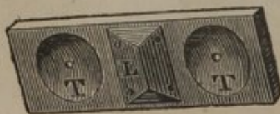
Fig. 2 affords a view of the lower side of the sliding shelf, in the wood of which it will be seen that there are two excavations, converging into two holes, one of which is seen at h , fig. 1.—This shelf is loaded with an ingot of lead at L, to prevent it from floating in the water of the cistern.
