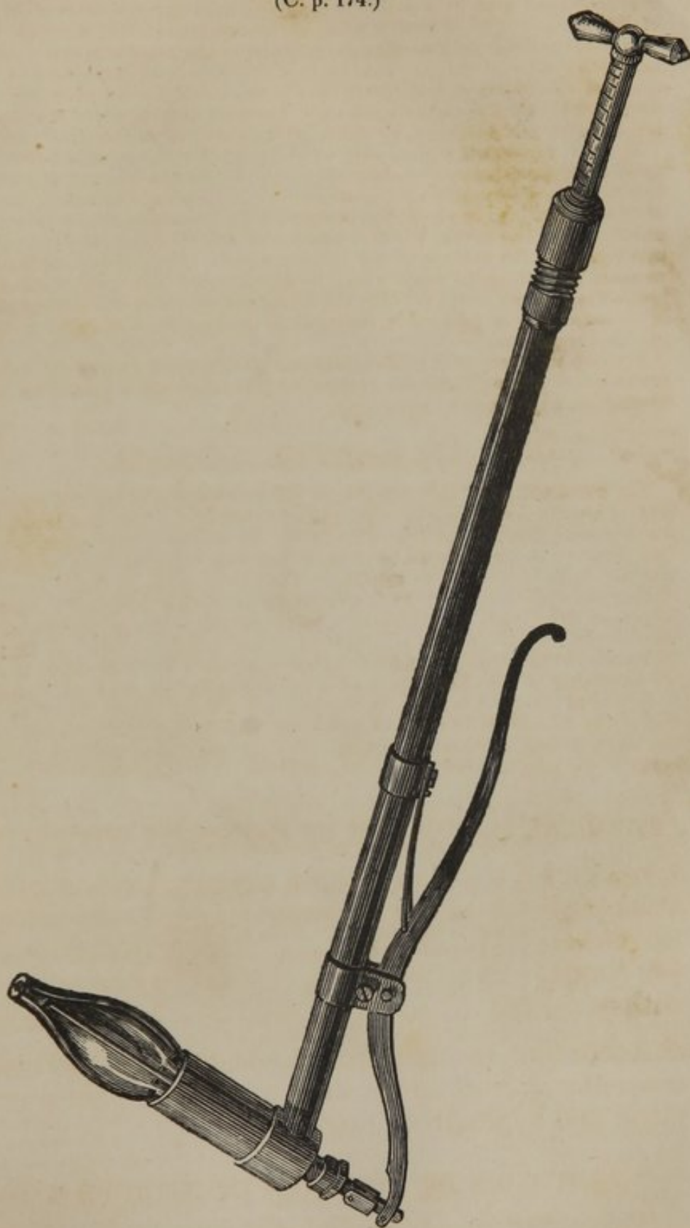
Sliding Rod Gas Measure. (C. p. 174.)
