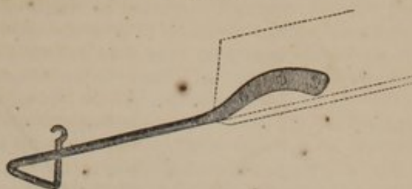
Bar of wrought iron for counter-extension.
