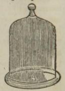
the receiver so firmly to the plate, that it requires a greater force than that of one man to remove it. In treating of the barometer, it is there shown that the atmosphere presses with a weight of 15lbs. upon every square inch of the earth's surface; therefore, supposing the surface of the receiver to contain only 36 square inches, the pressure of the atmosphere upon it is 36 multiplied by 15, or 540lbs. weight; but some allowance must be made for imperfect exhaustion.
