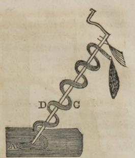
towards p, because it is situated higher above the horizon; and as this will always be the same in every similar part, it is evident that when the machine is in motion, the water, as it is raised by the spiral, will always remain on the under side till it flows out of the spout.
