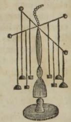
tive clappers, which are afterwards repulsed and driven off to the uninsulated bell in the centre, which receives their electricity, and conveys it through the bottom of the stand to the earth. Thus the five bells are kept continually ringing, which produces a pleasant peal when the tones of the bells are properly varied.
