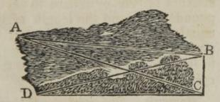
up with one third less power by crossing the road from A to B, than it would require in ascending directly from D to B. This is sufficient to show the great advantage loaded carriages obtain in ascending hills by crossing from one side of the road to the other; but here it must likewise be observed, as in every other part of mechanics, that what is gained by the power is lost in the time, inasmuch as the line A B is longer than D B.
