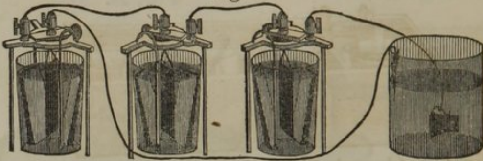
Fig. 34. Smee's Battery for Gilding and Silvering, (per pair.) Price $2.00.
