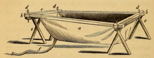
extended upon two long poles  $(b \ b)$ , passed through a broad seam on each side of the hammock, and kept asunder by the cross pieces (c), which are attached to the poles by the thumb screws  $(d \ d \ d)$ . At one end of the hammock is an air pillow, which can be readily blown up; and below it is a flexible tube (f), made of the same materials as the hammock, by which any water it may contain can be readily drawn off. When the poles are fixed, as in the above figure, and the open end of the
