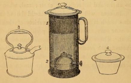
water-bath (1) placed over a lamp (2) in a wireworked cylinder; a small tin kettle (3) which enters the top of the cylinder; and a covered earthen-ware vessel (4) which fits into the waterbath; is useful for keeping fluids warm, and at the same time for preserving a light in the room, when an unshaded Lamp or a Candle would be hurtful.
