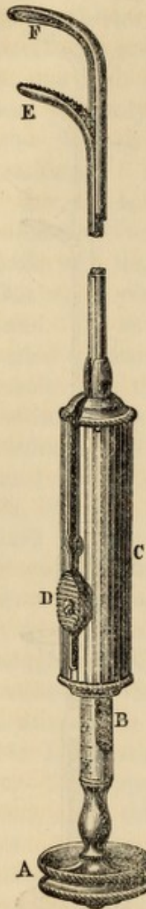
FIG. 40.—Lithotrite with cylindrical handle. A, Wheel-shaped end of sliding shaft, held in the operator's right hand, which directs the movements of the male blade E. B, The screw. D, The button which throws the screw into gear or releases it, as desired. C, The cylindrical handle attached by outer shaft to the female blade F.
