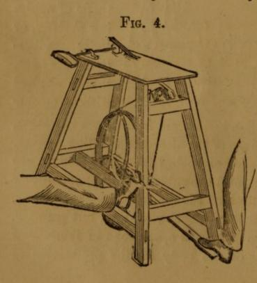
FIG. 4 will give an idea of the mechanical arrangement necessary to apply the above described forms of vibration. The foot of the operator acts upon a treadle, which turns a heavy wheel. This by means of a belt, turns rapidly a smaller wheel, whose axle has a crank or eccentric, which. by means of a connecting rod, gives the desired motion to the foot piece, or the hand piece, as the case may be.
