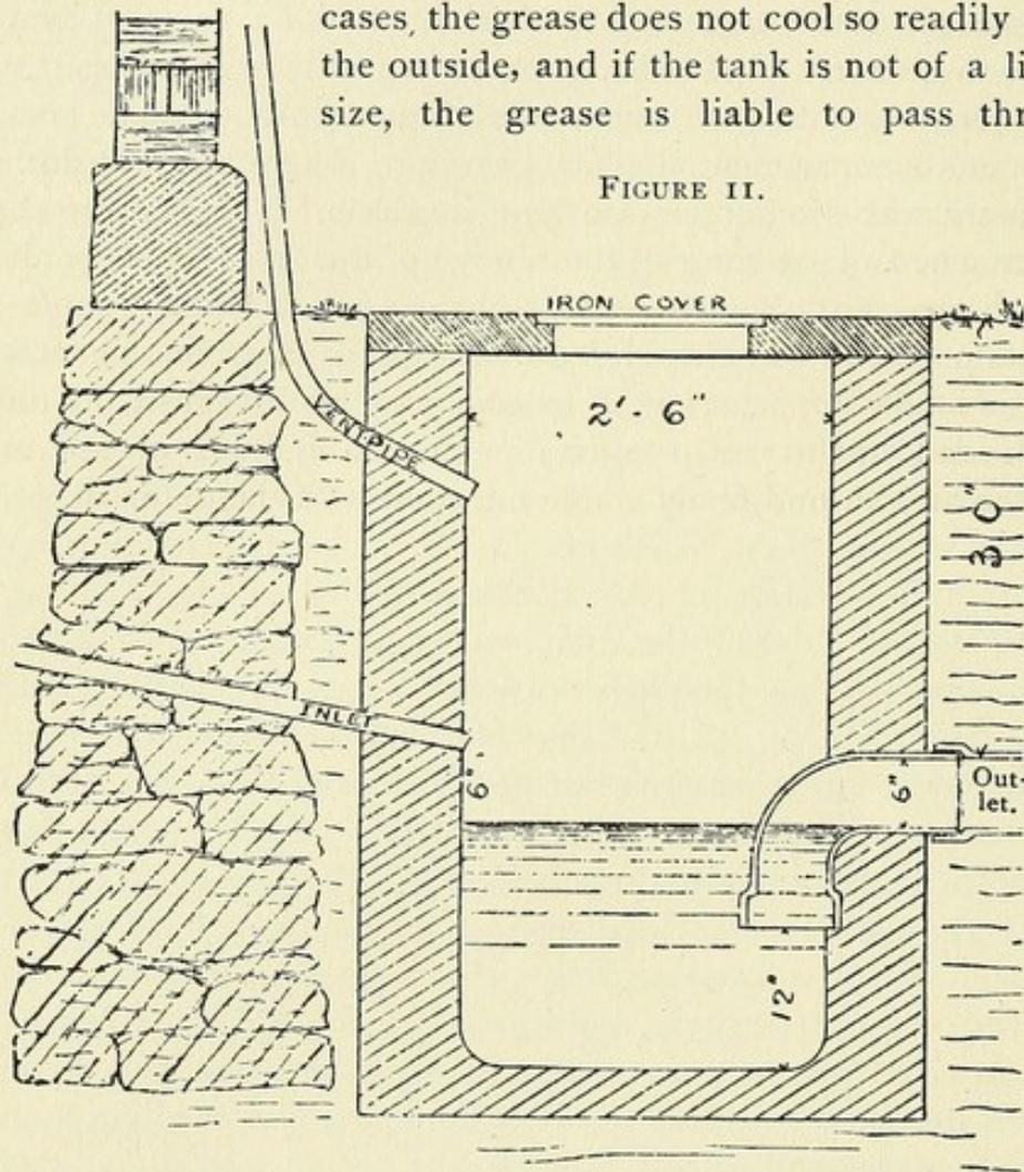
before being separated from the water. Whenever drains become choked with grease, if the pipe is accessible, it can be cleared by pouring hot water over the outside in a small stream, for half an hour or less. This heats up the whole contents, and the softened grease then passes along with the water that is applied inside. But the better way is to catch the grease before it gets into the pipes. If once allowed to coat the inner walls of the drains, much trouble will ensue.
