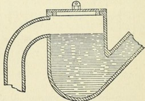
Its merits are that it requires a very strong blast of air through it to drive the water out and destroy the seal, so that this seldom happens. Moreover, the cleaning screw at the top enables one to readily get access to the interior for removing the sand or filth. This trap is often placed directly under floors, with the screw just visible through a hole in the floor for inspection and cleaning. Its faults are that it is a cesspool, though perhaps a small one, and soon
