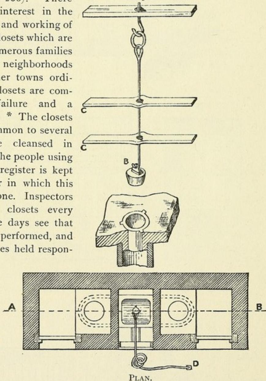
*B.—Enlarged Drawing of Valve, Guide Rod (C), &c.*
