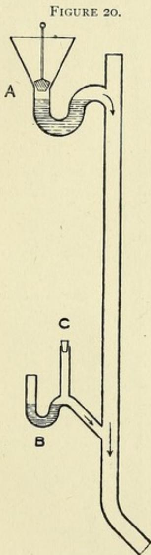
means of the glass test-tube, outside of the trap, that the water-seal is not disturbed this time. But if the vent-tube, instead of opening here at C, had been only one inch diameter or less, and some thirty feet long, with crooks in it, the air might have been so detained in it by friction that it would not have supplied the vacuum quickly enough to avoid disturbing the water-seal in this small trap.
