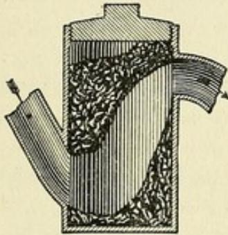
Housekeepers rarely, if ever, open these traps for cleansing. They are in out-of-the-way places, and are rarely thought of. The form with rounded bottom (Fig. 16—B) is more likely to keep clean than the flat bottom, which often accumulates filth, as shown in Figure 17.
