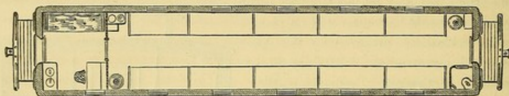
FIG. 5.—Horizontal section of the hospital cars on the Alexandria railway.
