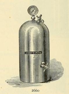
Fig. 2660-No. 7. This Receiver is made of copper, highly finished and plated. With first-class gauge, registering from one to fifty lbs. pressure; two accurately-fitted air cocks, and couplings for attaching the necessary rubber tubing.
